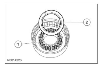
5. NOTICE: Do not fully compress the Clutch Spring Compressor or damage to the coast clutch piston spring retainer may occur.
