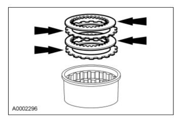
3. WARNING: While removing or installing the retaining ring, slowly release tool pressure on clutch piston springs. Failure to follow this instruction may cause the assembly to separate forcefully, resulting in serious personal injury.
