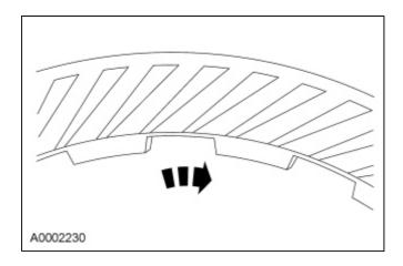
7. Install the 2 steel clutch plates and 2 friction clutch plates in alternating order starting with a steel clutch plate.
