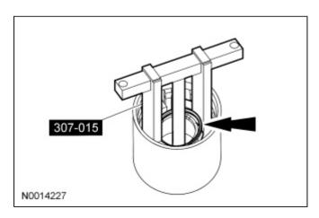
6. *NOTICE:* Coast clutch friction plates are directional and must be installed with grooves clockwise (ID to OD). The word TOP should face up, otherwise transmission damage can occur.
